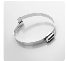
Master-Grip Hose Clamp, screwable, Steel quality W4, stainless steel 1.4301 Special clamp for fastening light and medium-weight, right-handed spiral hoses such as Flamex B-se, Flamex B-F se, Master-PUR Trivolution, Master-PVC and Master-SANTO
