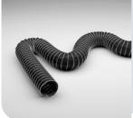
Suction & Blower hose made from VITON<sup>®</sup>coated Polyester fabric, for corrosive media up to +210 °C, electroconductive, surface resistance ≤ 10<sup>4</sup> Ohm
